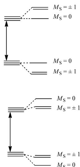
Figure 6. Interaction scheme between the ground and first triplet excited states through the  $z$  components of spin-orbit operator that couples  $M_S$  levels of the same values and stabilizes the  $M_S = \pm 1$  components (top), and interaction between the ground and the second excited triplet states through the  $x$  and  $y$  components of the spin-orbit operator that couples states with different  $M_S$  values and stabilizes the  $M_S = 0$  component (bottom).
