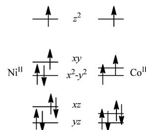
Figure 5. Orbital energy diagrams for **1** (left) and **2** (right).
