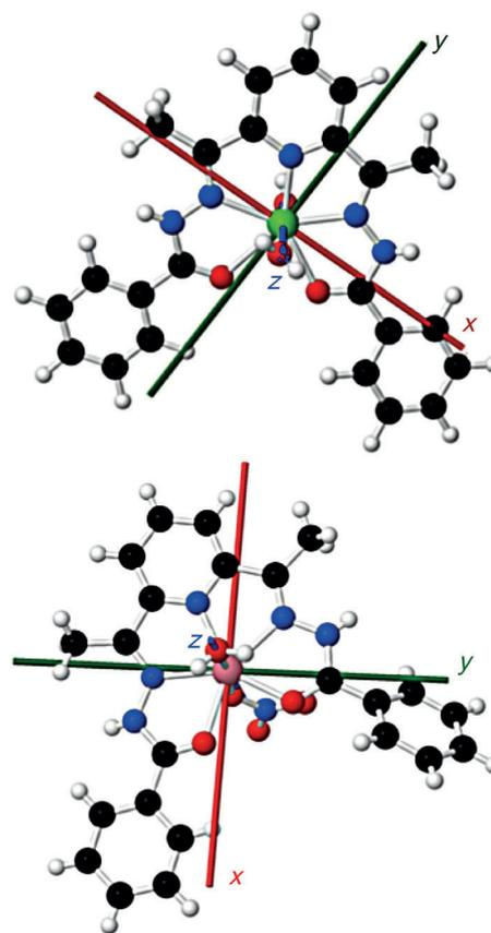
Figure 7. View of the magnetic axes obtained from ab initio calculations. For **1** (top), the magnetization is along  $z$  (negative  $D$ ), and for **2** (bottom), the magnetization is in the  $xy$  plane (positive  $D$ ).
