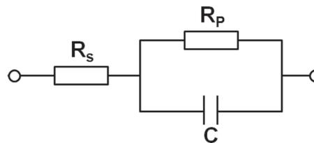
**Figure 4.** Equivalent circuit applied to model the experimental capacitance behavior.
