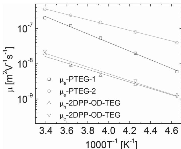
**Figure 8.** Mobility of charge carriers versus temperature for PTEG-2, PTEG-1 and 2DPP-OD-TEG (symbols) and corresponding Arrhenius fit (lines) yield the activation energies ~0.2 eV.
