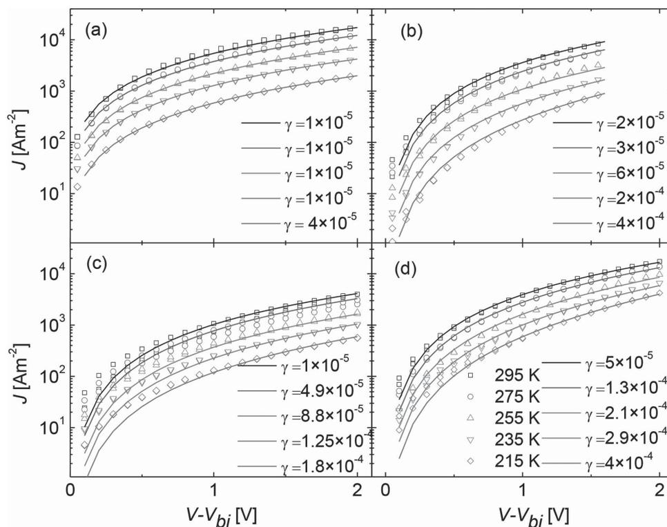
**Figure 7.** Steady state current voltage corrected for  $V_{bi}$  of a) Al/PTEG-2(192 nm)/Al, b) Au/PEDOT:PSS/PTEG-1(145 nm)/LiF/Al, d) Al/2DPP-OD-TEG(80nm)/Ba/Al electron-only devices and c) Au/PEDOT:PSS/2DPP-OD-TEG (96 nm)/MoO<sub>3</sub>/Al hole-only device at temperatures ranging from 295K-215K in 20 K steps. Data (symbols) are fitted with Equation (4) (lines). The gamma values ( $\gamma$  [V m<sup>-1</sup>]<sup>1/2</sup>) for each fit are provided in the legend.
